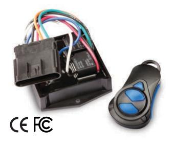
Warner Linear's wireless actuator control can be used to remotely control a 12 or 24VDC actuator up to 100 ft. away. It can be used with our standard line of P1 end limit controls. The unit is offered in a single and dual actuator output for the 12VDC unit. The 24VDC unit is only available with two actuator outputs. All models have a manual override feature to operate the actuator without a remote. The wireless system is an RF design operating at 915MHz.
